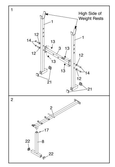
Be sure that the Uprights (1) are oriented as shown; the high side of the weight rests must be on the indicated side. Attach the Frame (2) to the Crossbar (3) with two M8 x 55mm Bolts (14), two M8 Washers (12), and two M8 Nylon Locknuts (13). Do not tighten the Nylon Locknuts yet.
